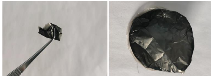
Fig. S6 Images of LDHT flexible film absorbers
