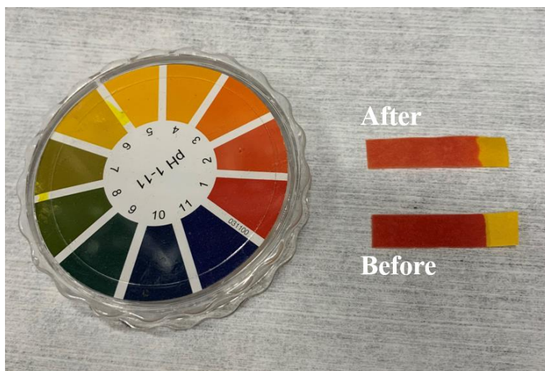
Fig. S1 pH value of the CBD-SnO 2 precursor solution after heating at 95 °C for 3 hours (as depicted in Fig. 1b, Step ②)
