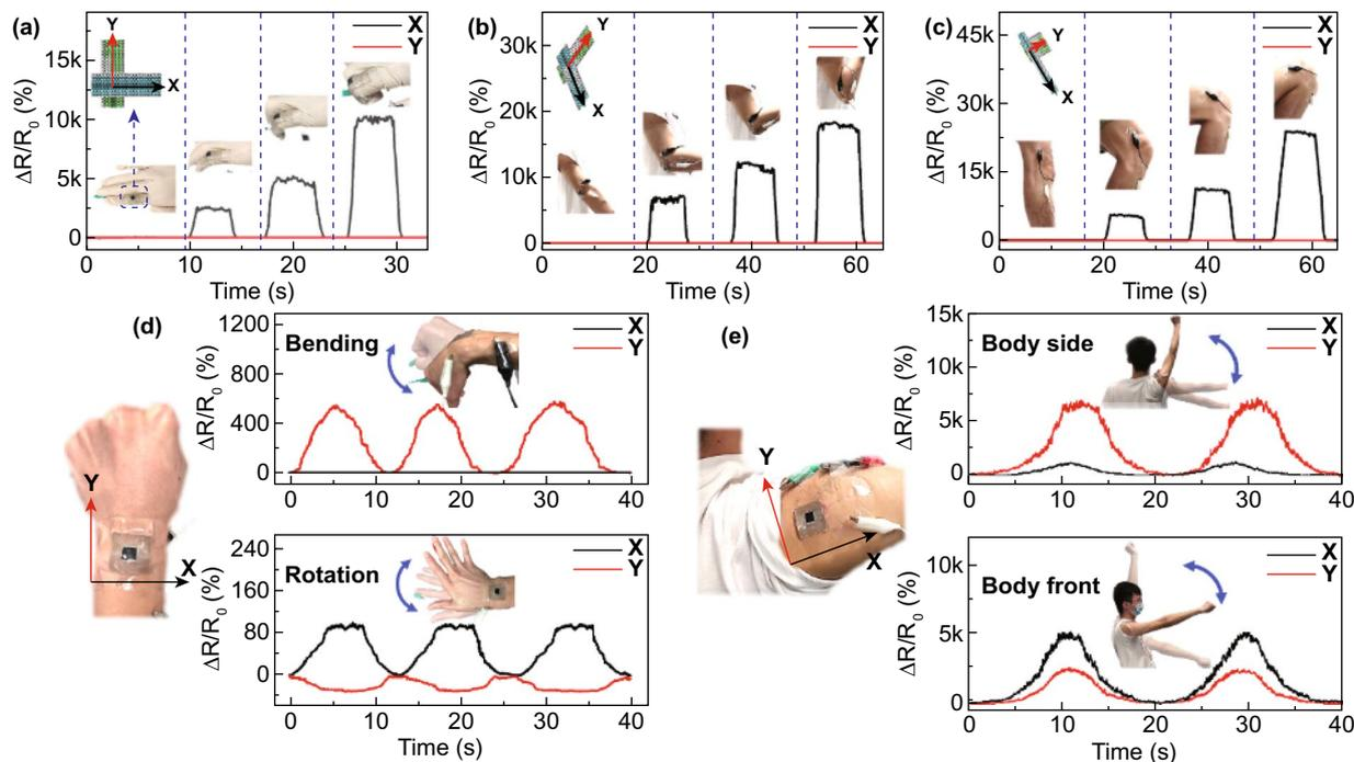
**Fig. 5** Demonstration of full-range strain sensing of complex human motions by the multidirectional sensor. Detection of bending of **a** finger, **b** elbow, and **c** knee joints to different degrees. Detection of multiaxial movements of **d** wrist and **e** shoulder joints
