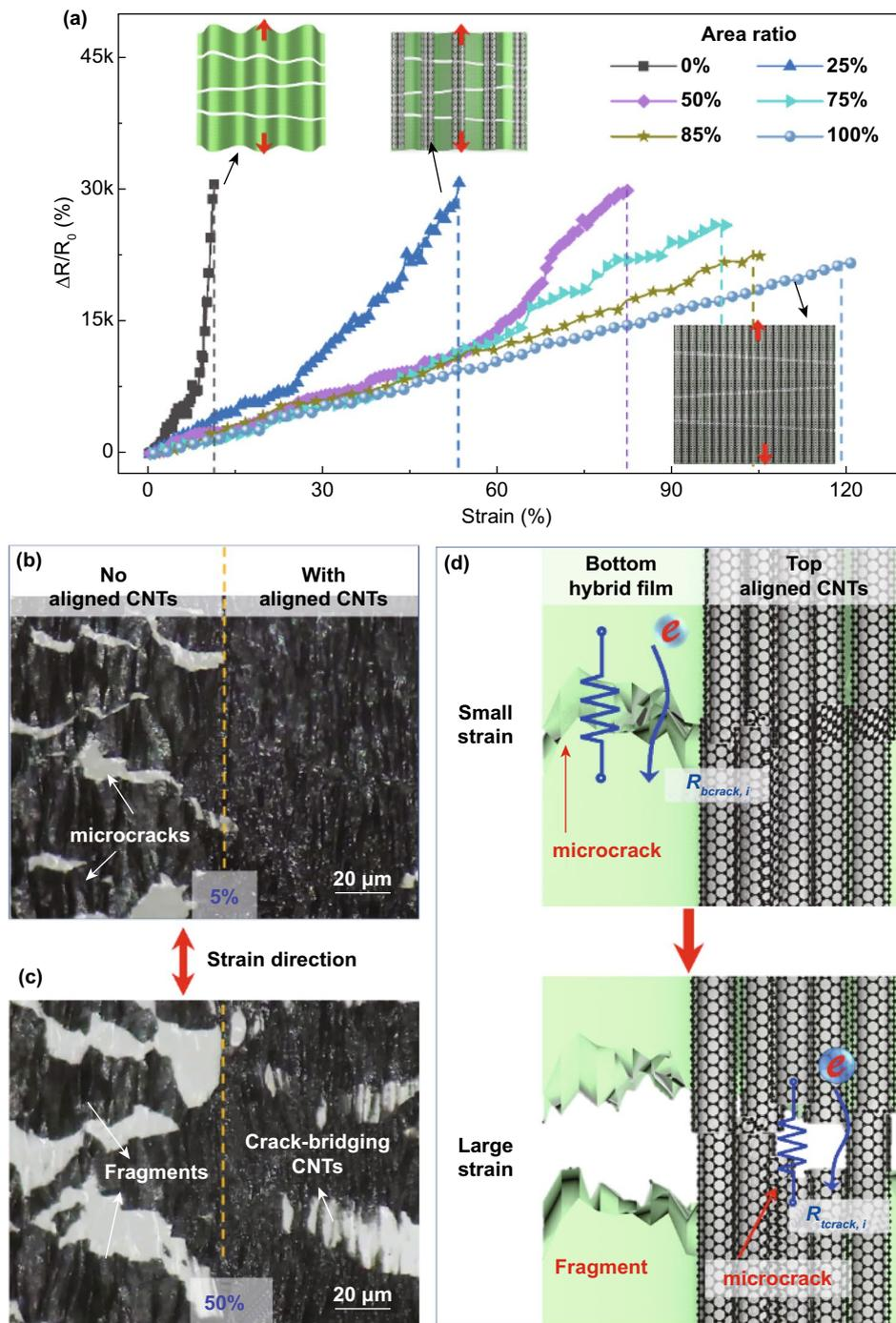
**Fig. 2** Optimization of stretchability and linearity of the sensor. **a** Relative resistance changes in T-direction of bilayer sensors with different area ratios of top to bottom films: schematics of the corresponding structures in inset. Morphologies of bilayer sensors when loaded at **b** 5% and **c** 50% strains in T-direction. **d** Schematic illustration of stepwise crack propagation mechanism
