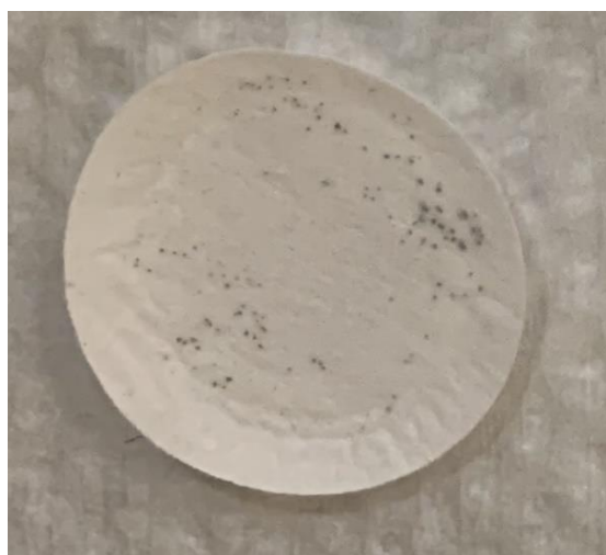
Fig. S7 Photograph of the pristine separator of Zn|Cu cell after short-circuit
