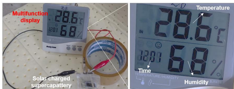
Fig. S7 Powering multifunction electronic display by solar charge solitary supercapattery
