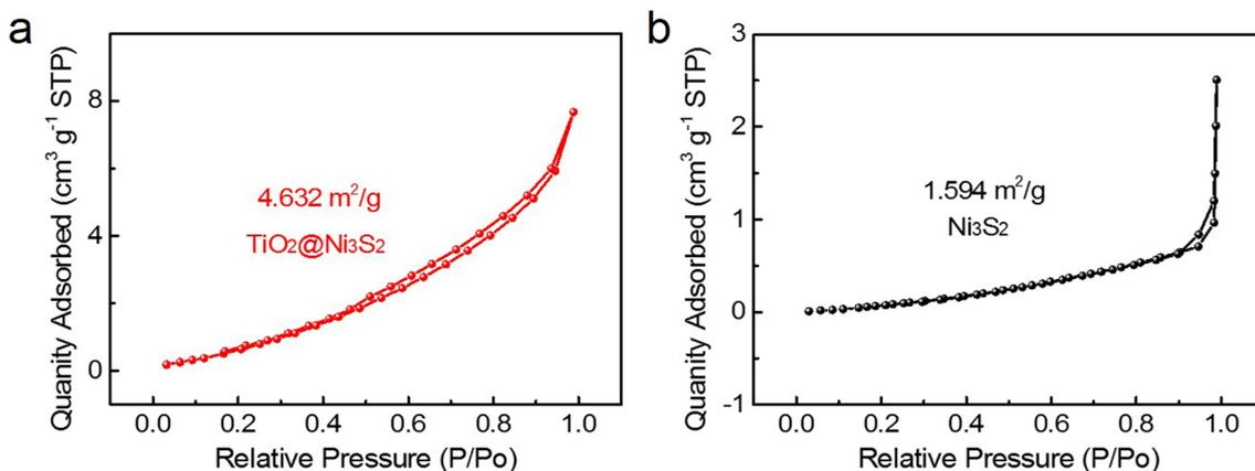
**Fig. S4** BET measurements: nitrogen adsorption-desorption isotherm curves: **a**  $\text{TiO}_2@Ni_3S_2$  nanowire arrays and **b**  $Ni_3S_2$  arrays
