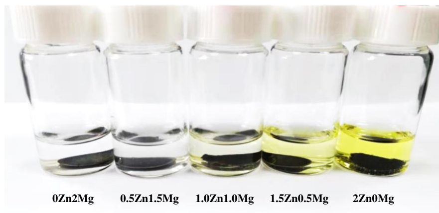
Fig. S13 Optical image of the MgVO electrodes in different electrolytes for 24 h. With the increase of MgSO 4 concentration, the dissolution of active material is effectively controlled
