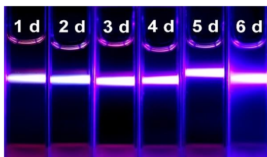
Fig. S4 Tyndall effects for structural stability of PAA 68 - b -PEG 86 - b -PAA 68 /MnO 2 (1 mg mL -1 ) in DMEM with FBS (10%, v/v) for 6 days
