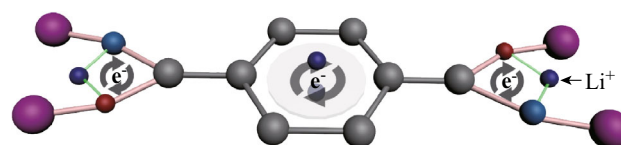
Scheme 2 The schematic view of lithiation sites for \text{Li}^+ adsorbed on benzene ring and amide group with the electron-donating effect of Co-BDCN-24h
