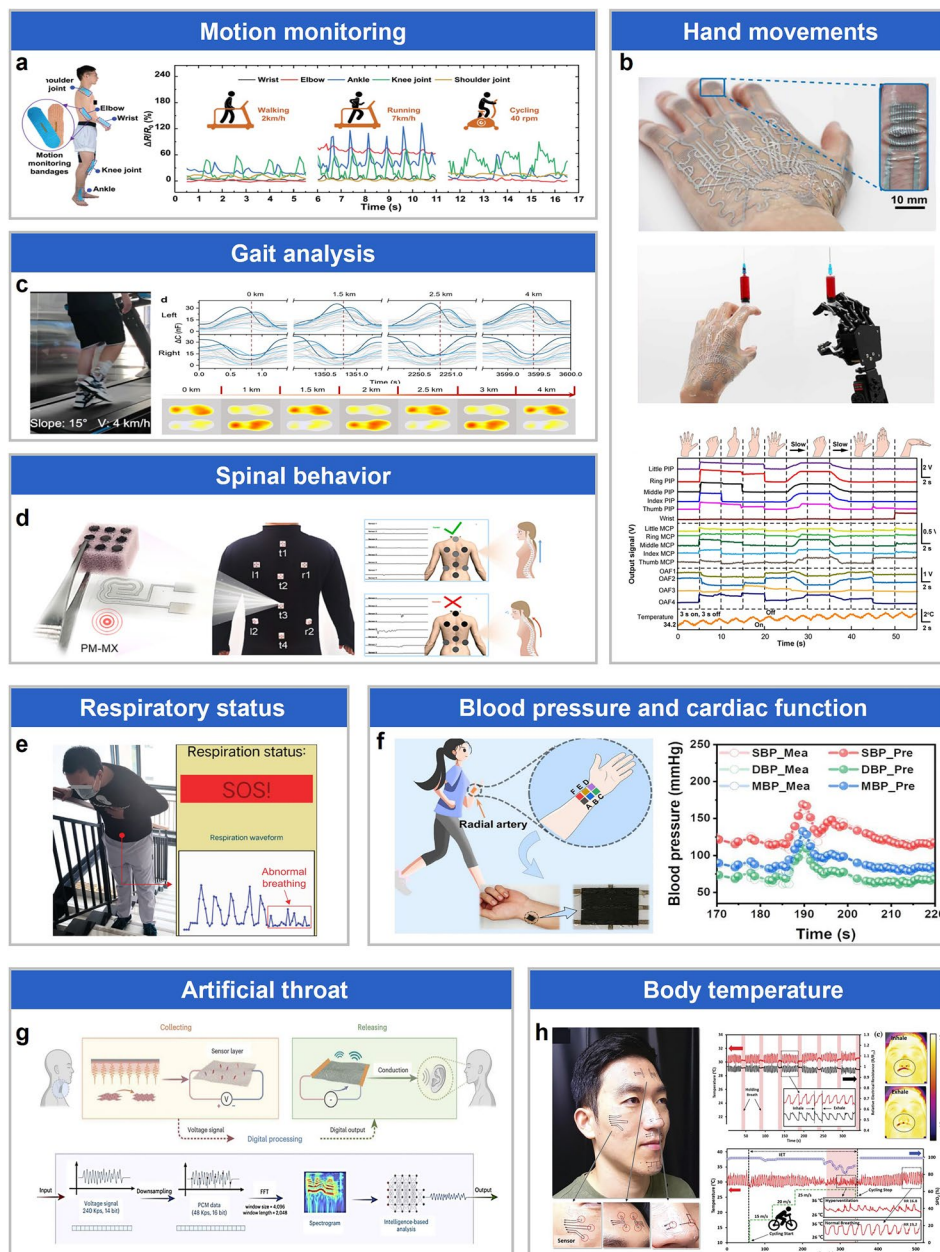
Fig. 11 On-skin epidermal electronics for physio-physiological recording. a Epidermal Fabric Strain Sensors for motion monitoring for sports. Reproduced with permission [150]. Copyright 2023, Wiley–VCH. b On-skin METT for real-time recoding of different hand movements. Reproduced with permission [152]. Copyright 2021, American Association for the Advancement of Science. c Integrated iontronic flexible pressure sensor for human plantar pressure and gait analysis. Reproduced with permission [153]. Copyright 2024, American Chemical Society. d Dual network piezoresistive sensor for spine behavior monitoring. Reproduced with permission [156]. Copyright 2024, Elsevier. e Wearable health-care system based on fiber strain sensors for monitoring respiratory status. Reproduced under terms of the CC-BY license [158]. Copyright 2024, National Science Review. f Wearable strain sensor array for real-time blood pressure and cardiac function monitoring. Reproduced with permission [159]. Copyright 2023, American Association for the Advancement of Science. g Speech interaction paradigm based on the wearable artificial throat. Reproduced with permission [160]. Copyright 2023, Springer Nature. h Conformal epidermal temperature sensor for respiration sensing. Reproduced under terms of the CC-BY license [162]. Copyright 2019, Wiley–VCH
