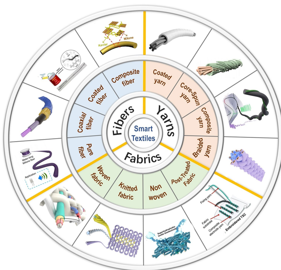
Fig. 1 Schematic diagram of the classification and preparation methods of smart textiles: Pure fiber, Reproduced with permission [38]. Copyright 2020, Springer Nature. Coaxial fiber, Reproduced with permission [39]. Copyright 2022, American Chemical Society. Coated fiber, Reproduced with permission [40]. Copyright 2015, John Wiley and Sons. Composite fiber, Reproduced with permission [41]. Copyright 2024, The American Association for the Advancement of Science. Coated yarn, Reproduced with permission [42]. Copyright 2021, John Wiley and Sons. Core-spun yarn, Reproduced with permission [43]. Copyright 2021, American Chemical Society. Composite yarn, Reproduced with permission [44]. Copyright 2021, Royal Society of Chemistry. Braided yarn, Reproduced with permission [45]. Copyright 2022, Elsevier. Woven fabric, Reproduced with permission [46]. Copyright 2022, Springer Nature. Knitted fabric, Reproduced with permission [47]. Copyright 2022, Springer Nature. Nonwoven, Reproduced with permission [48]. Copyright 2022, Elsevier. Post-treatment. Reproduced with permission [49]. Copyright 2024, John Wiley and Sons
