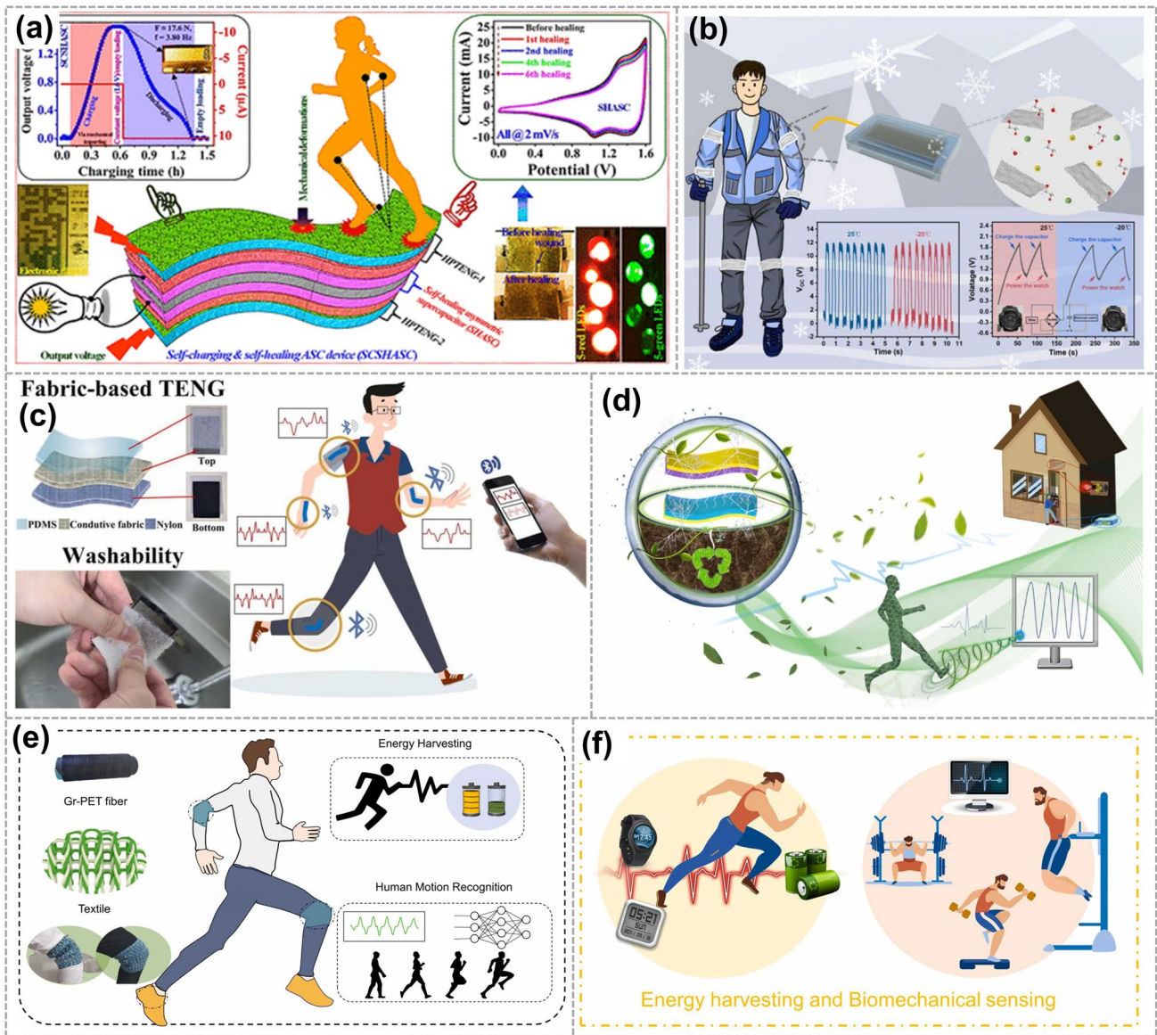
Fig. 11 Graphene electrode-based TENG is used for human body monitoring. a TENG-driven self-charging and self-healing flexible asymmetric supercapacitor power cell. Reproduced with permission. Reference [101] Copyright 2019, American Chemical Society. b Anti-freezing and stretchable TENG based on liquid electrode for biomechanical sensing in extreme environments. Reproduced with permission. Reference [102] Copyright 2022, Elsevier. c TENG was applied to four positions on the human body for sensing movement. Reproduced with permission. Reference [51] Copyright 2021, Elsevier. d A fully degradable TENG is used for monitoring human motions. Reproduced with permission. Reference [103] Copyright 2023, Elsevier. e Schematic diagram of diversified applications enabled by the 3D textile TENG. Reproduced with permission. Reference [104] Copyright 2022, Elsevier. f Schematic diagrams showing the application of the stretchable porous MXene/LIG foam-based TENG in human motion energy harvesting. Reproduced with permission. Reference [105] Copyright 2022, Elsevier
