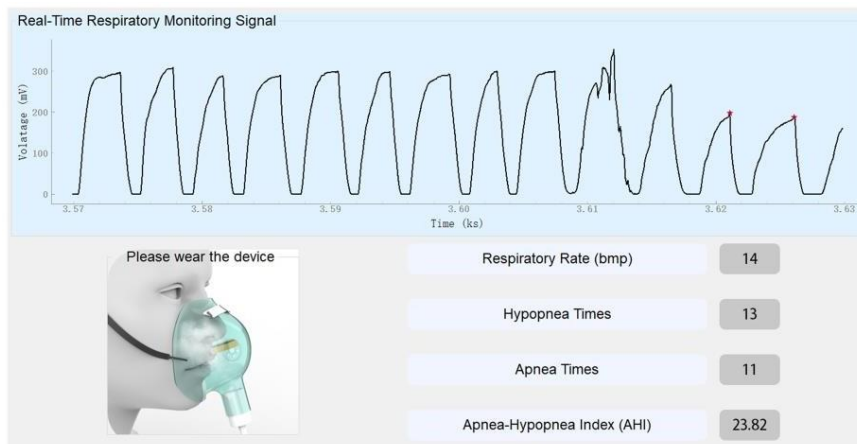
Fig. S40 Real-time monitoring of respiration by the OSAHS diagnostic system for one hour. The experiment was carried out on Apr. 25, 2022, in Beijing, China, with a 40% RH
