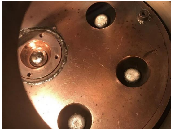
Fig. S1 Image of the arc melting furnace cavity
