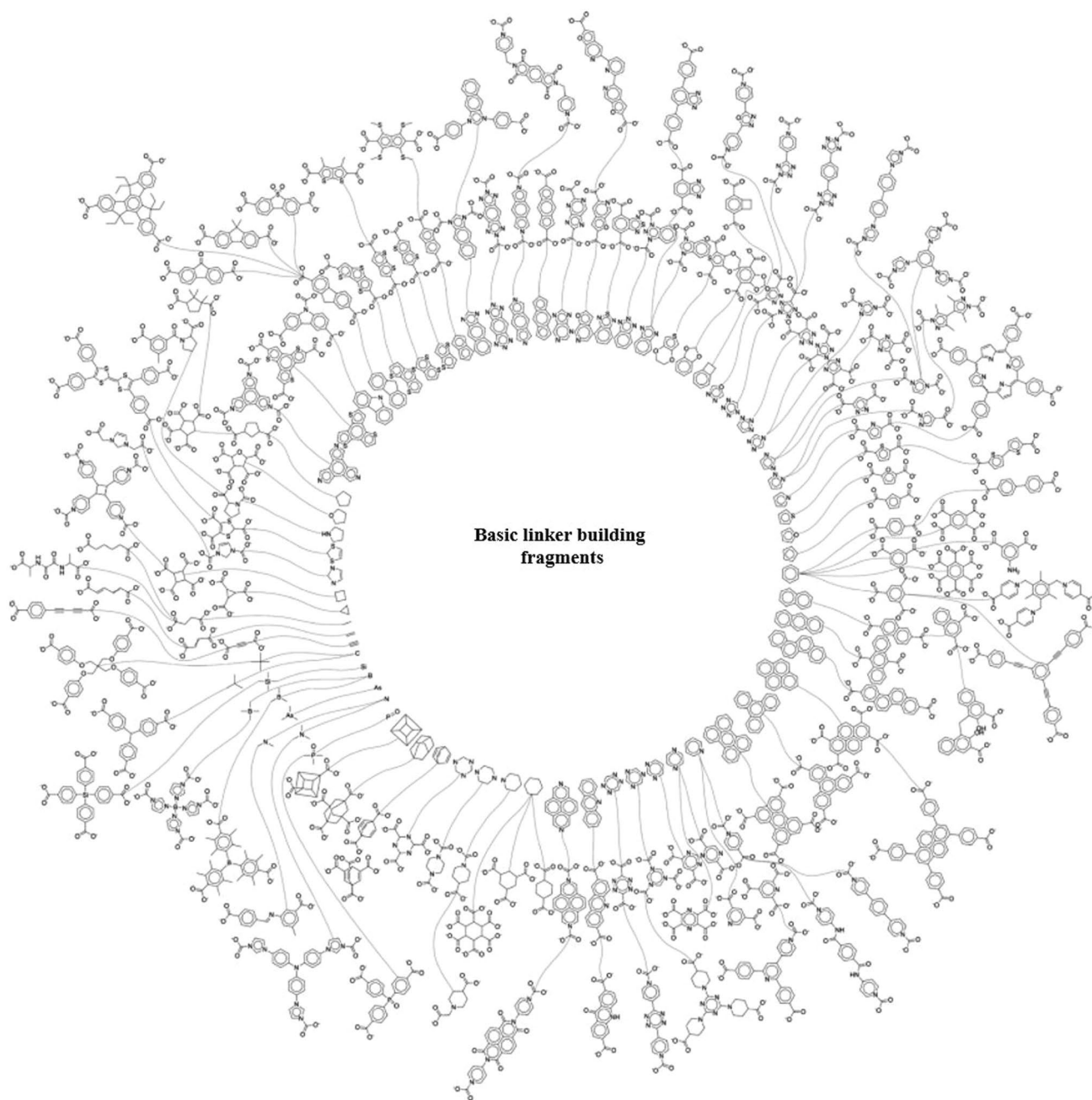
Fig. 6 Power of ligand diversity. An analysis was carried out on the linkers present in all reticular framework structures from the CoRE database. The results of this analysis have been represented in a scaffold tree plot, which highlights the basic building fragments of the latest RF-NPs that have a high occurrence rate. These building fragments are depicted in the inner circle of the plot. The second and third circles of the plot illustrate the linkers that have been derived from these building fragments. The plot provides a comprehensive visual representation of the linkers and building fragments present in state-of-the-art RF-NPs, which can be useful for further research in this field. Reproduced with permission from Ref. [74]. Copyright 2021, Springer Nature
