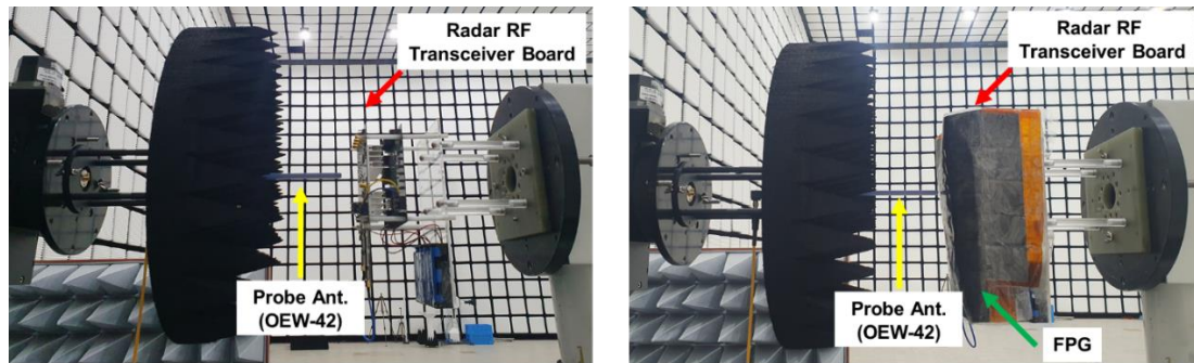
Fig. S2 Experiment environment to measure 2-dimensional electric field distribution of radar RF board without FPG and with FPG
