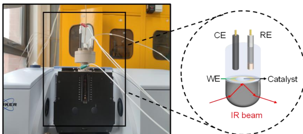
Fig. S10 The schematic diagram of in situ ATR-FTIR tests
