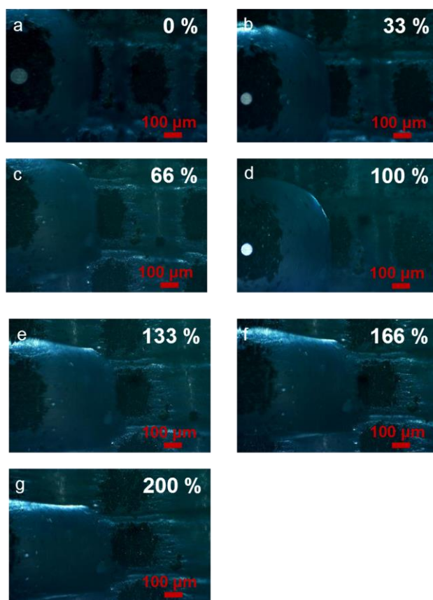
Fig. S6 Change of the contact angle along with the film stretching. a-g Optical photographs of the stretched water drop at strains from 0% to 200%
