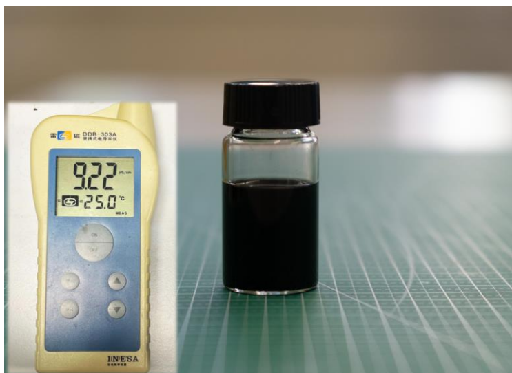
Fig. S2 Optical image and solution conductivity of the MXene/CNTs ink
