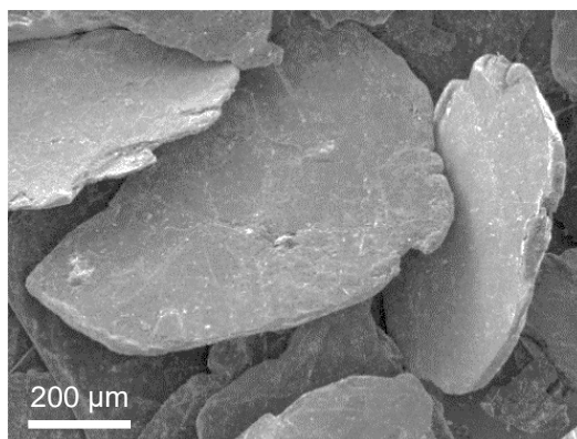
Fig. S2 SEM image of the used flake graphite
