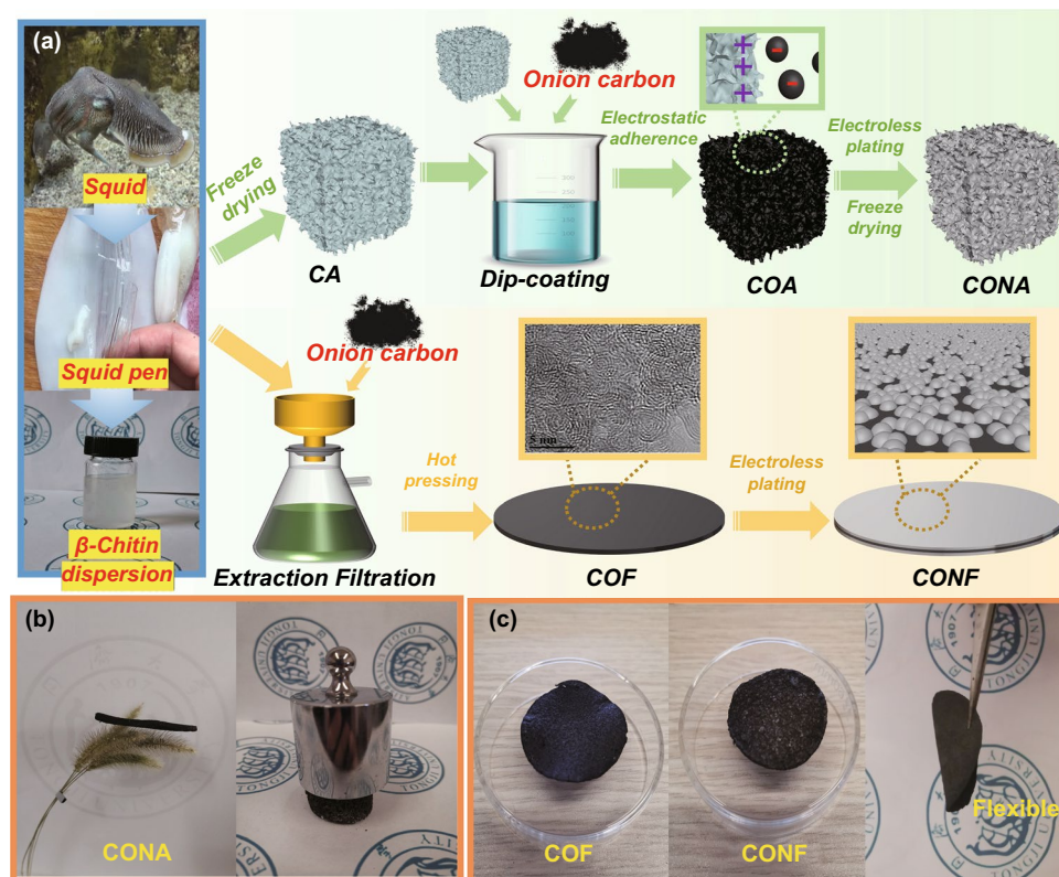
Fig. 1 a Schematic illustrating the synthetic processes of CONA/CONF; b digital images exhibit the CONA standing on dandelion and compression resistance performance; c digital images display flexible COF and CONF
