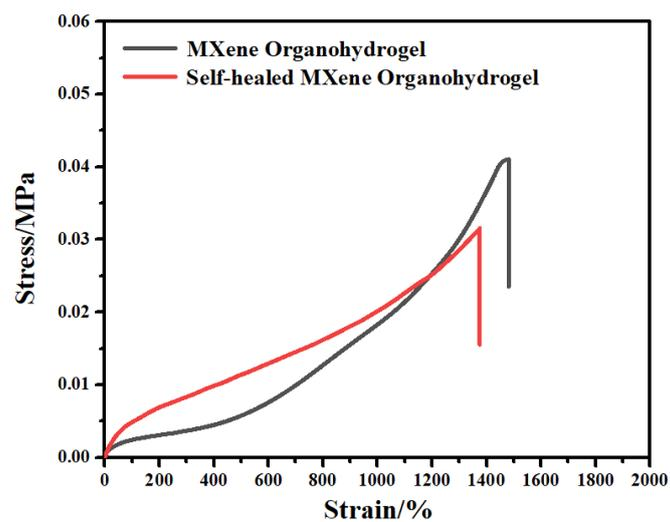
Fig. S8 Stress-strain curves of original and self-healed MXene organohydrogels.
