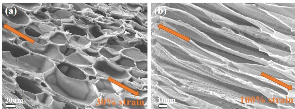
Fig. S14 SEM images of freeze-dried MXene organohydrogels (MXene content of 0.4 wt%, Gly displacement time of 30 min) under (a) 30% and (b) 100% strains.
