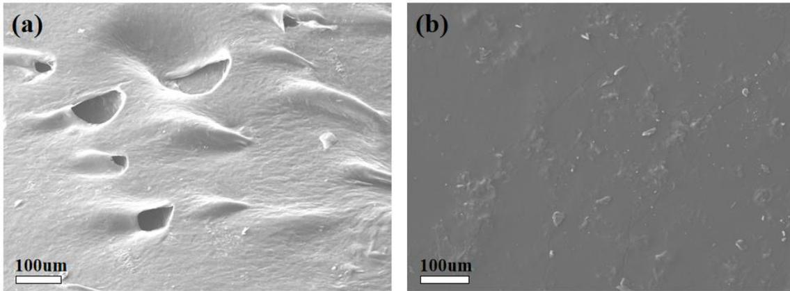
Fig. S9 SEM images of (a) MXene hydrogel stored for 7 days and (b) MXene organohydrogel stored for 7 days.
