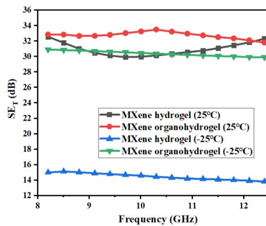
Fig. S13  $SE_T$  curves of MXene hydrogel and MXene organohydrogel before and after freezing.
