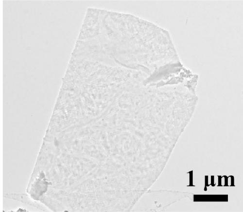
Fig. S2 TEM image of MXene nanosheet.
