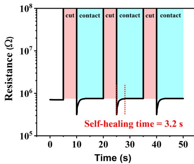
Fig. S7 Change of resistance of MXene organohydrogel during several self-healing processes.
