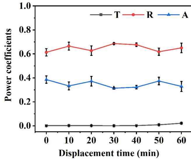
Fig. S11 The absorption (A), reflection (R) and transmission (T) coefficients of MXene organohydrogels with different water-Gly (1:1) displacement time.
