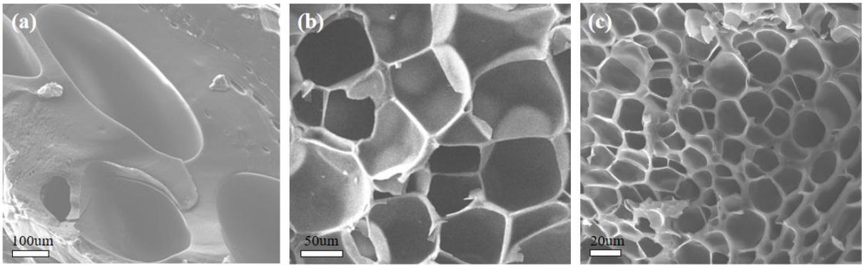
Fig. S4 SEM images of (a) pure hydrogel, (b) MXene hydrogel with MXene content of 0.4 wt%, and (c) MXene hydrogel with MXene content of 2.2 wt%.
