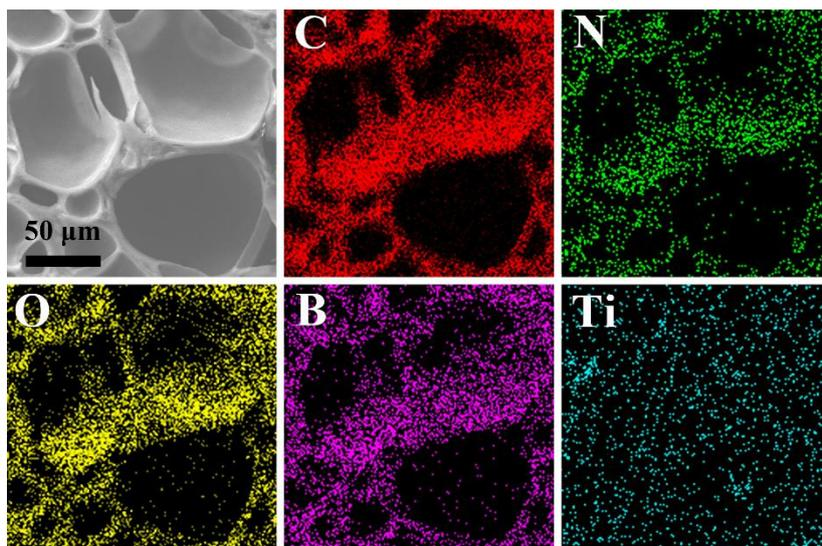
Fig. S3 SEM and elemental mapping images of MXene hydrogel (MXene content of 0.4 wt%).
