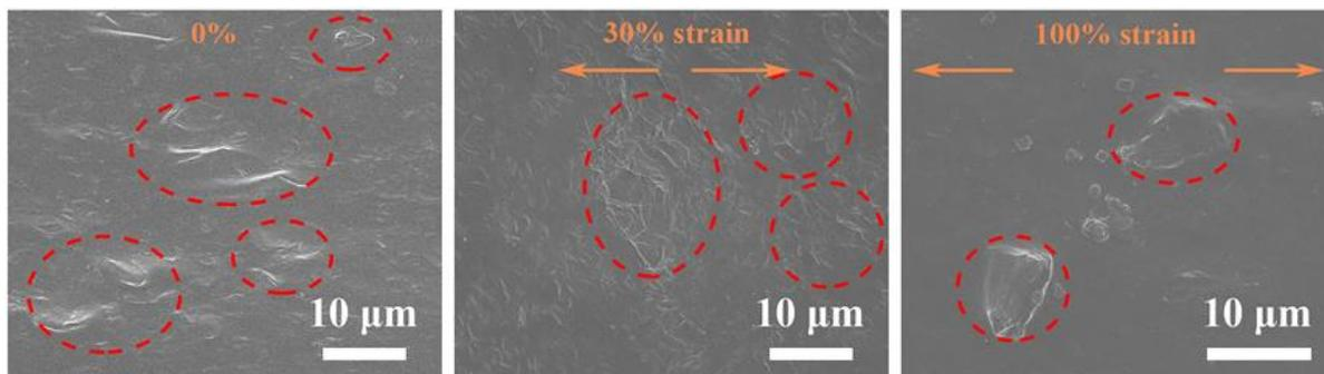
Fig. S15 SEM images of MXene organohydrogel under 0%, 30% and 100% strains.
