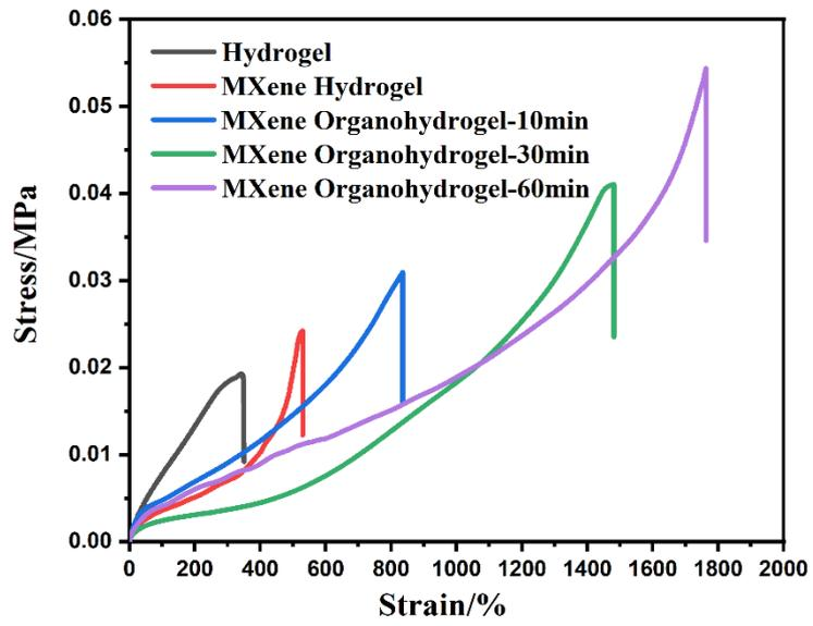
Fig. S6 Stress-strain curves of pure hydrogel, MXene hydrogel and MXene organohydrogels.
