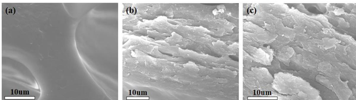
Fig. S5 High magnification SEM images of (a) pure hydrogel, (b) MXene hydrogel with MXene content of 0.4 wt% and (c) MXene hydrogel with MXene content of 2.2 wt%.
