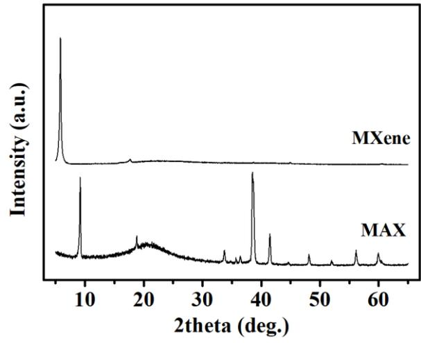
Fig. S1 XRD patterns of MAX powder and MXene nanosheets.
