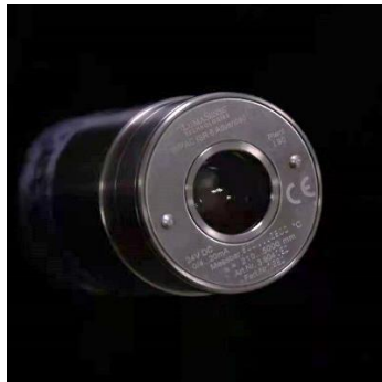
Fig. S18 Photograph of infrared thermometer (ISR 6 Advanced, LumaSense IMPAC)
